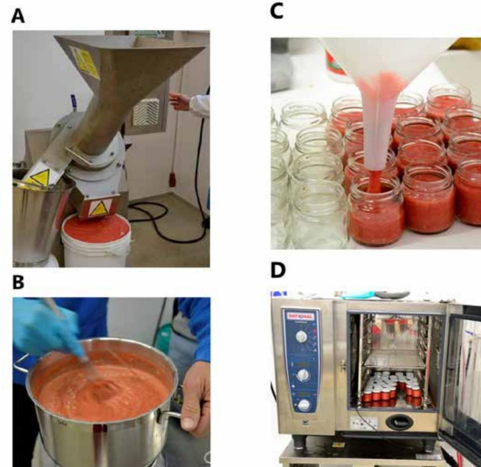
Fig. 1: Processing steps for fruit spread production: (A) Production of puree; (B) Production of fruit spread; (C) Hot canning; (D) Pasteurization at 85 °C.
