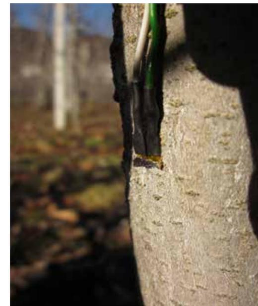
Fig. 1: A temperature sensor prior to (left) and after insertion (right) under the tree bark. The red arrow indicates the sensor's exact measuring point.
